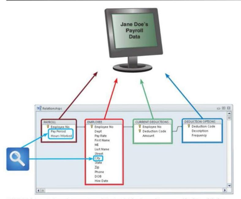
FIGURE 1-6 In a typical payroll system using a relational model, data is stored in separate tables that are linked to form an overall database.
